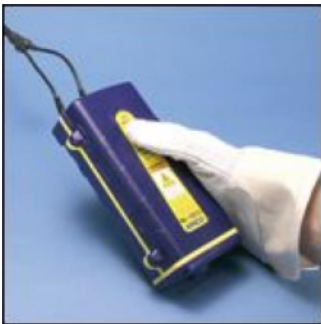
Step 3 Press and hold Control Unit switch and wait for ignition.
